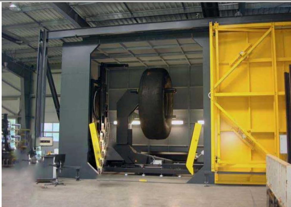
Figure 5. OTR and GOTR vacuum shearography machine with a seat diameter of up to 63" manufactured by "Steinbichler" (Germany), model "Intact 4300-3, in the Povolzskaya Tire Company
